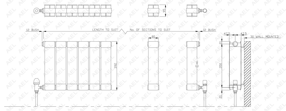
AEL HEATING SOLUTIONS FARAL SILL LINE (FF) FLAT FRONT ALUMINIUM RADIATORS FF3-100
