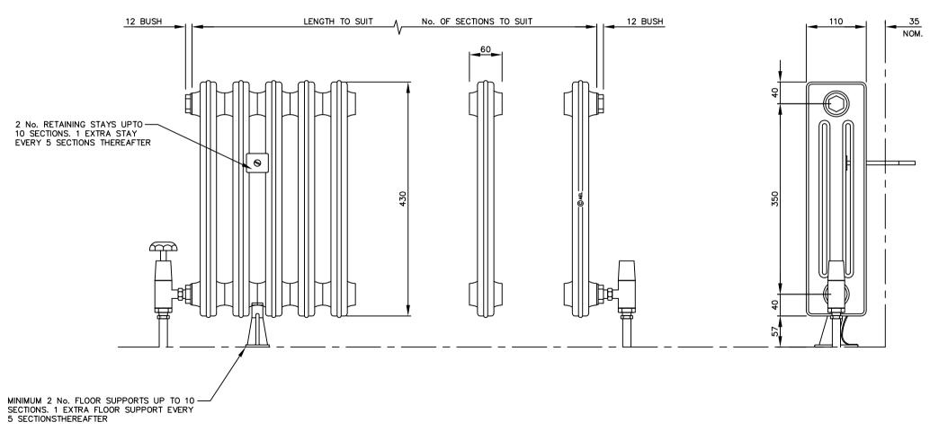
AEL HEATING SOLUTIONS VISCOUNT CAST IRON RADIATOR K110 / 43
